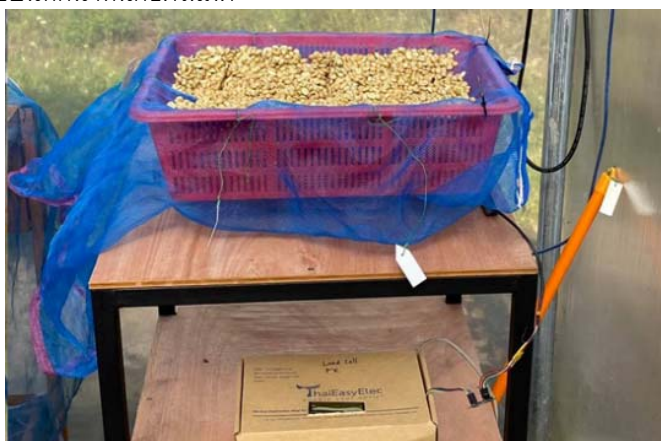
Figure 1 Automatic data logging scales
